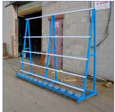
Vertical Transfer Conveyor w/ Donut Rollers
