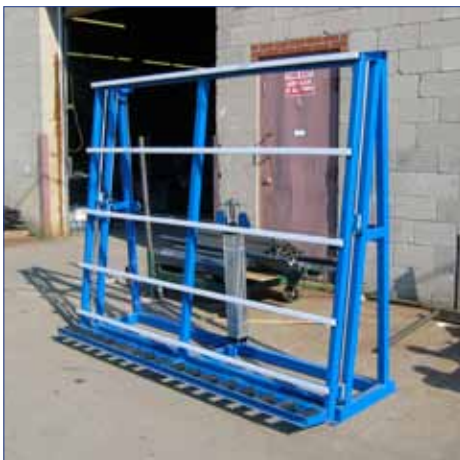
Vertical Transfer Conveyor w/ Pneumatic Lift
