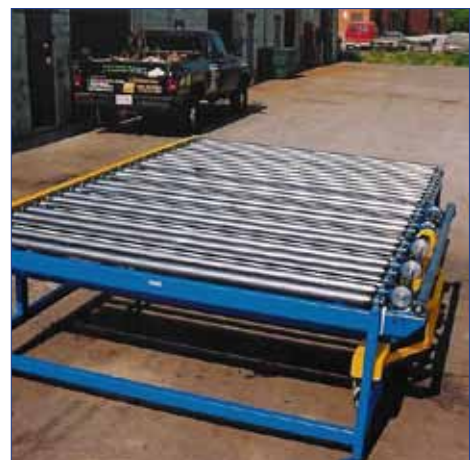
Power Corner Conveyor
