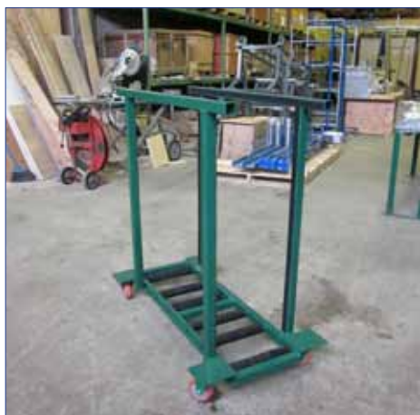
Movable Conveyor Bridge & Dolly
