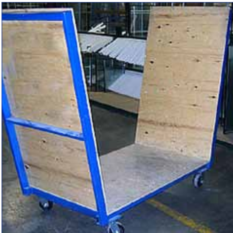
Completed Window Dollies
