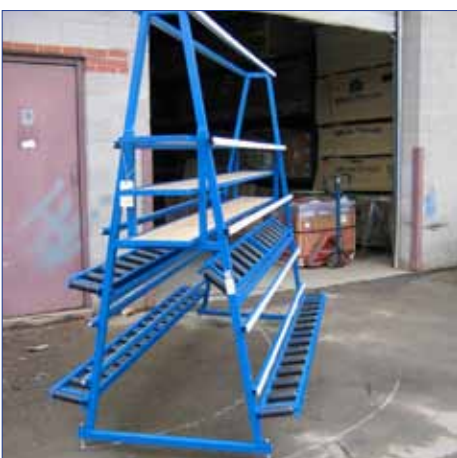
Double-Sided Vertical Transfer Conveyor with Multiple Ledges
