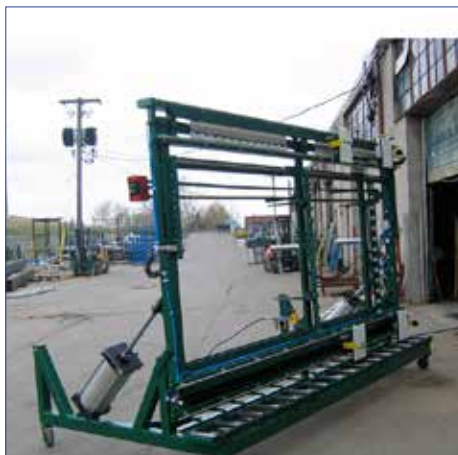
Oversized Door Assembly Rack with Pneumatic Tilt
