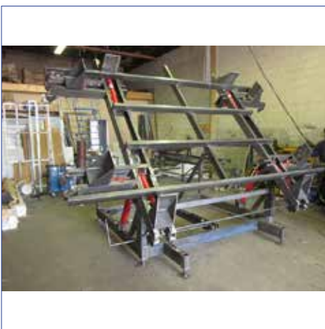
Heavy Duty Hydraulic Tilt Table
