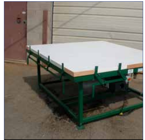
Grid Application Table with Air Float
