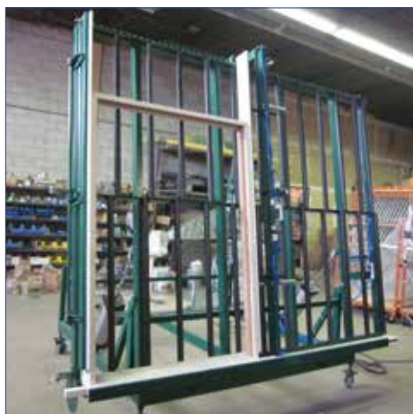
Pneumatic Tilt Clamping Table w/ Rollers
