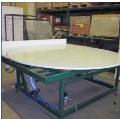
Rotating Work Table w/ Pneumatic Tilt
