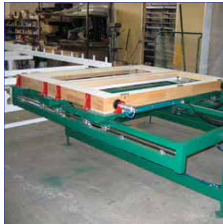
Tilting Assembly Table with Clamps
