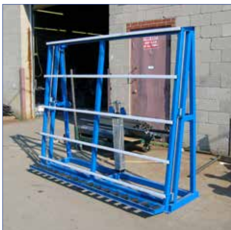
Vertical Transfer Conveyor w/ Pneumatic Lift
