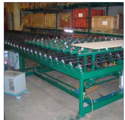
Load/Off-Load Conveyor w/ Pop-up Casters
