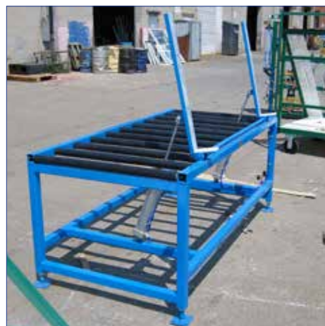
Roller Table with Pneumatic Flip-Up Finger
