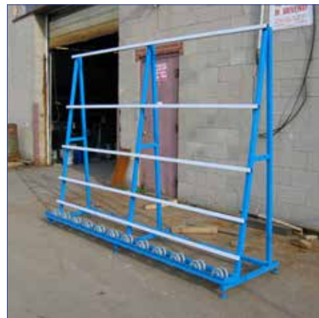
Vertical Transfer Conveyor w/ Donut Rollers
