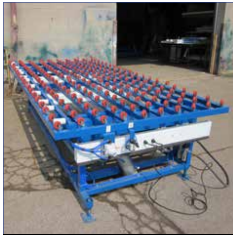
Glass Inspection Table with Pneumatic Tilt
