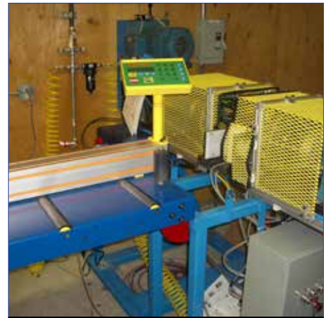
TigerStop on a 2-Head Drilling Machine
